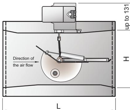
**Ref. no. 504:** Similar to ref. no. 503, additional auxiliary switch for activation of an additional switching command.
