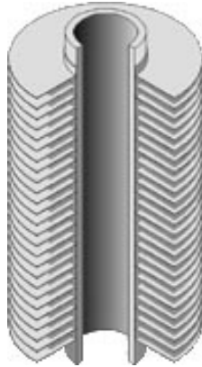
Figure 42 – 5/8" (16 mm) Tension-Wound Finned Tubing 10 Fins per Inch
